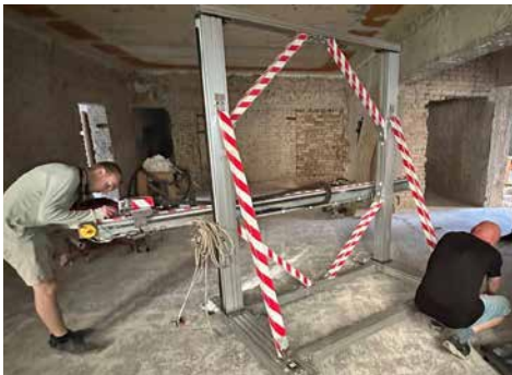
Yan Kormilitsyn and fellow students prototyped a 3D printer to recycle the rubble of buildings that were hit by Russian attacks in Kyiv.
